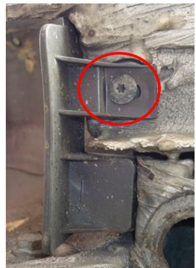
Figure 2 Adapter screws underside of body
