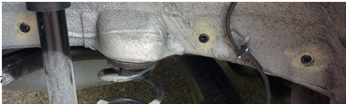
Figure 8 Inner arch chassis holes with 3 screw inserts N908 338 01 fitted each side
