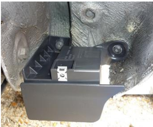
Figure 5 New adapter screw in place using the existing screws
