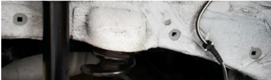
Figure 7 location of the inner arch chassis holes
