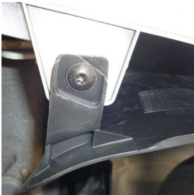
Figure 13 Rear liner fitting to existing bodywork
