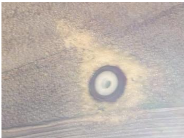
Figure 9 Outer arch chassis hole with screw inserts N 106 213 01 fitted
