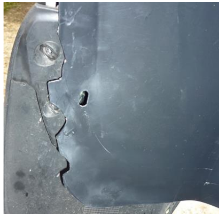
Figure 11 Area to trim for mud flap fitting
