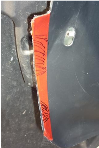
Figure 12 Liner showing area to trim
