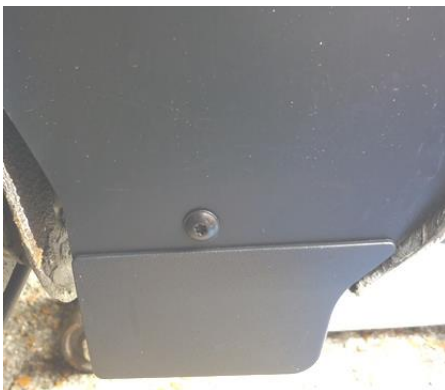
Figure 6 Liner front edge fits into adapter slot and is screwed in position
