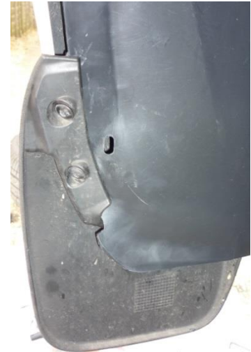
Figure 10 Liner fitted between mud flap and mud flap clip
